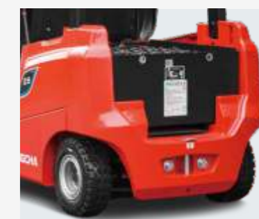
Battery is placed at the rear of the truck
